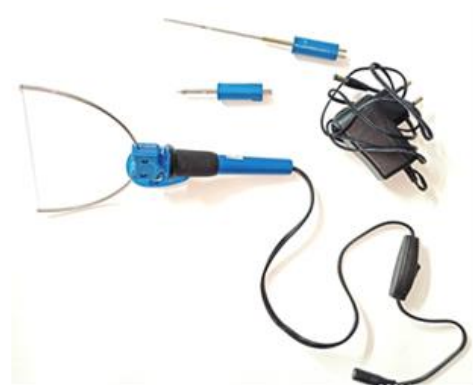
Figure 9: Circle/Compass Cutter [source: author]
