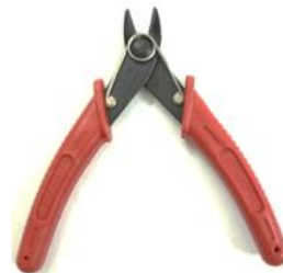
Figure 10: Wire Cutter [source: author]
