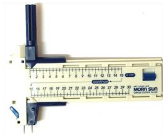
Figure 8: Circle/Compass Cutter [source: author]
