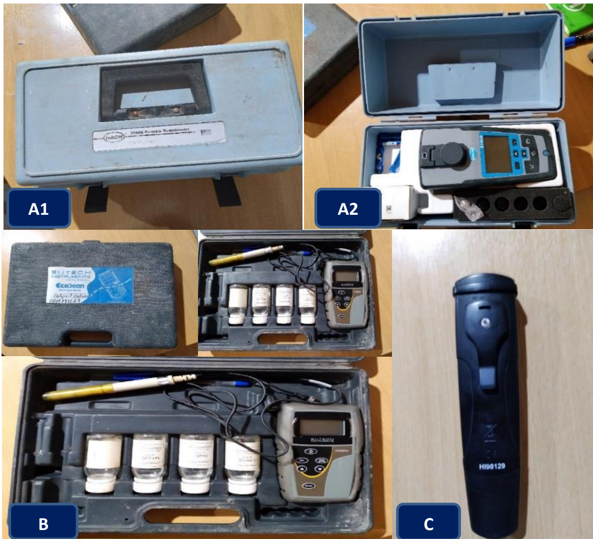
Figure 1: Photos of Instruments used this study, (A1 & A2), is turbidity tester, (B), is Electrical conductivity tester and (C) is TDS and EC tester.
